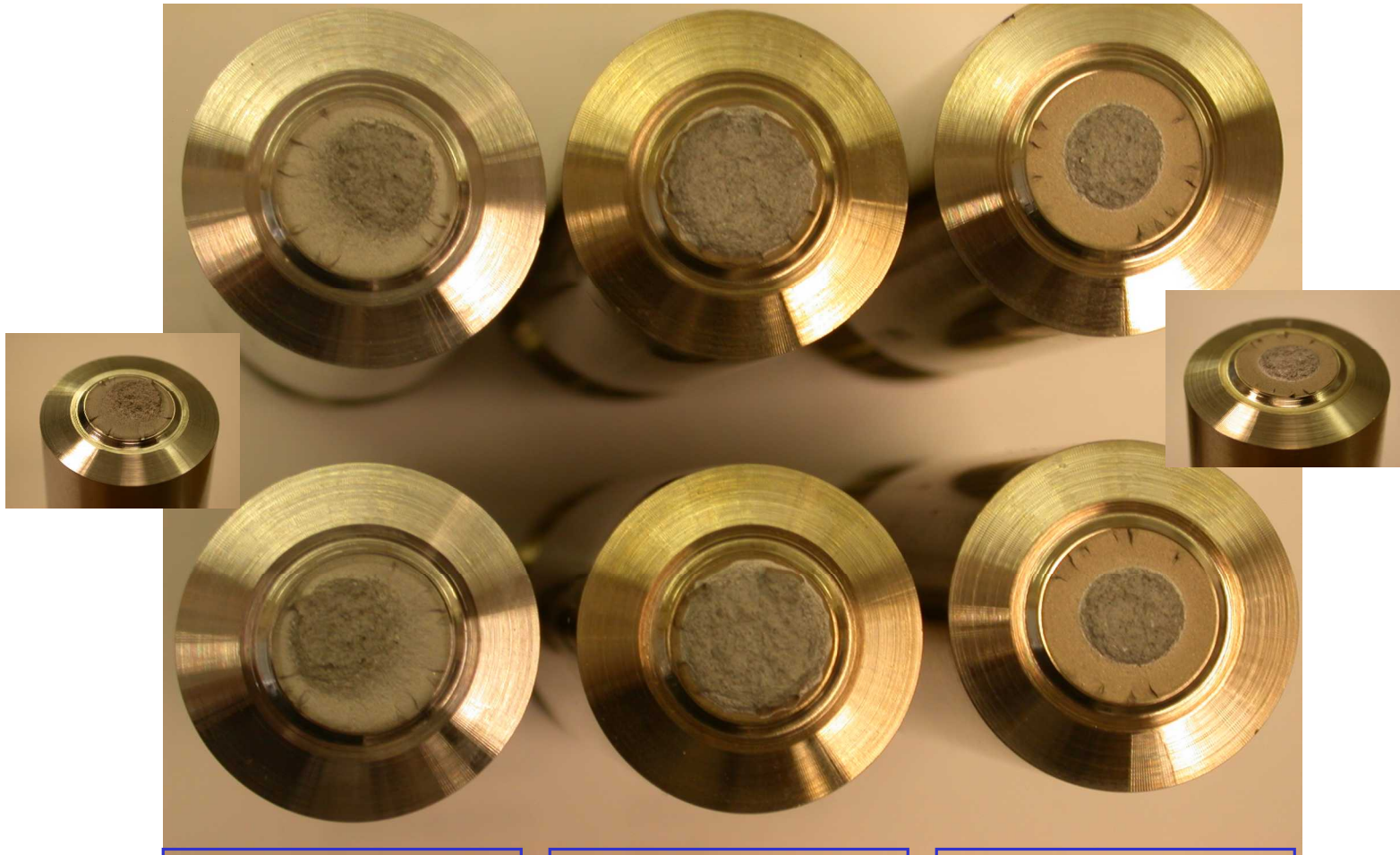
Asymmetric precracked specimen a/r \approx 0.7
