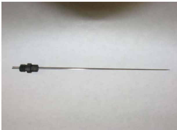
Figure 5. Four pictures of the components which make up the two different anode rod holder assemblies. (1) W rod friction fit into the graphite holder to be used with both the existing and modified holder assembly, the OD of the graphite holder is threaded. (2) W rod and graphite holder screwed into the 3 piece stainless steel rod holder assembly. (3) 3 piece stainless steel assembly broken out with attaching screws also shown W rod inserted into graphite holder. (4) W rod and graphite holder screwed into Al rod holder flush to the Dome. Not shown graphite holder sticking out.
