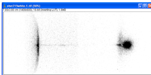
Figure 14. Cygnus1 white pinhole camera using the standard stainless steel holder with graphite section of holder assembly flush.
