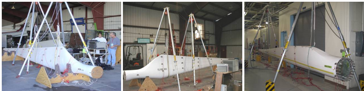
Figure 5. Photos of Modal Tests Performed on the Blades in Figure 4. (a) CX-100 (left), (b) TX-100 (center), (c) BSDS (right)
