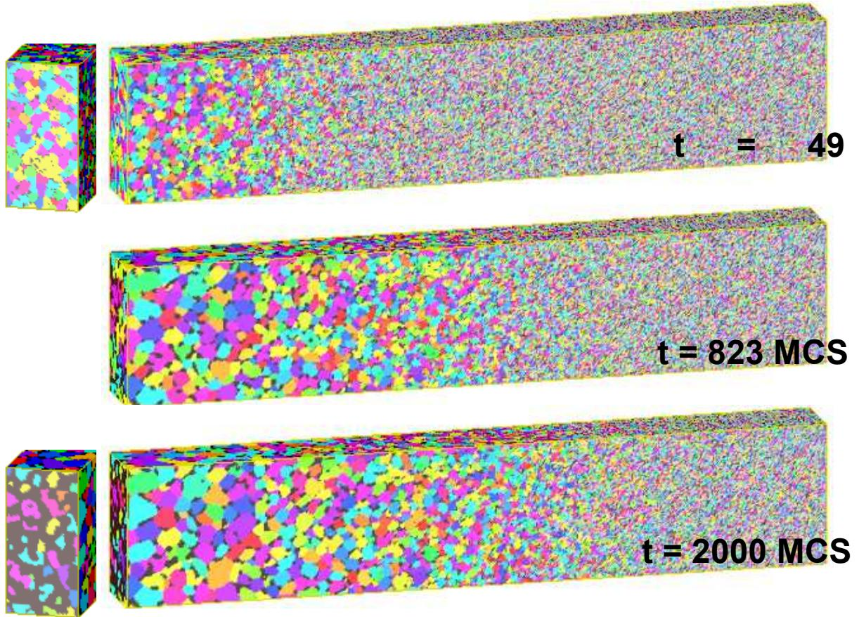
bubbles towards the high-temperature side as shown in the side view at the left side. Early in the simulation at time  $t = 49$  MCS, the bubbles are homogeneously distributed through out the sample. However, at time  $t = 2000$  MCS, the bubbles are diffusing toward the high-temperature side. The bubbles have become large and connected and grains are poking into the bubbles.
