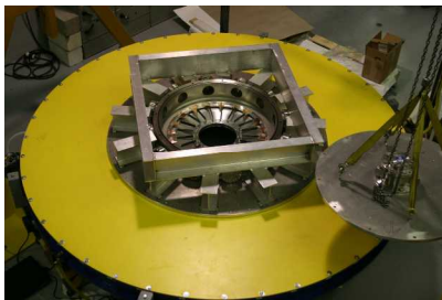
Resistive load in Vacuum chamber Filled with \text{SF}_6
