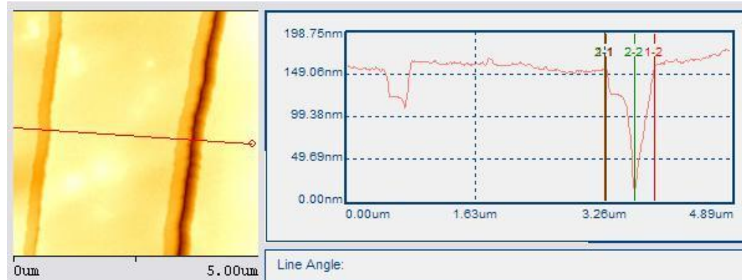
Measurement of crack width and depth from AFM image
