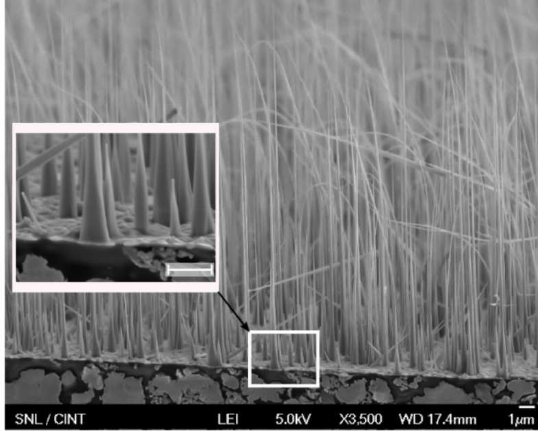
Figure 3. SEM photograph of \sim 15 \mu\text{m} long InAs nanowires grown on a Si:GaAs(111)B substrate.
