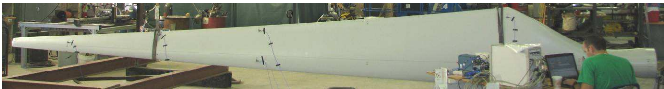
Figure 2: Experimental setup for modal test of sensorized rotor blade with free boundary conditions.
