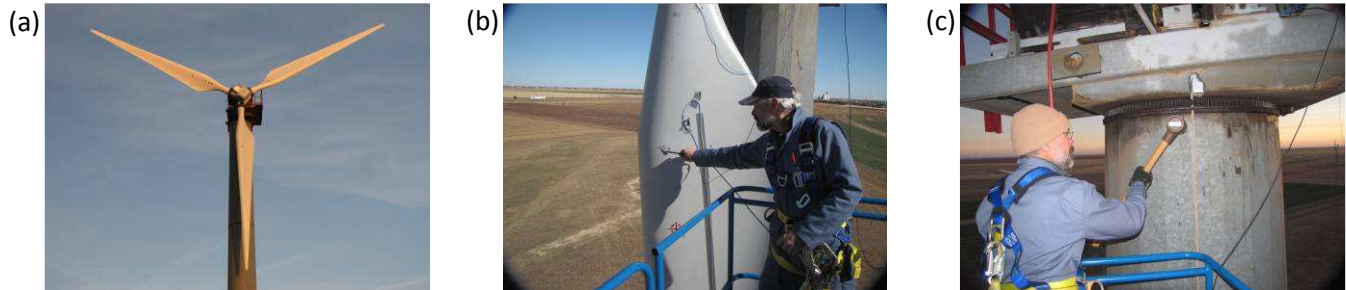
Figure 4: (a) Micon 65/13 Wind Turbine with the Sensored Rotor Blade mounted. (b) Modal impact testing of the wind turbine rotor blades. (c) Modal impact testing of the wind turbine tower.
