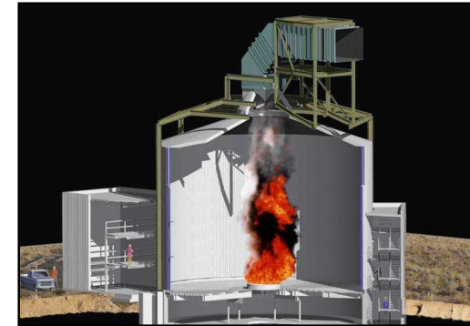
Test conducted in Flame Test Cell at Sandia using 3 m burner
