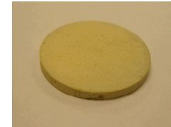
50 wt% AgI/50 wt% Glass A, 500 °C for 3 hr
