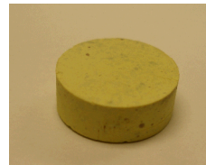
20 wt% AgI- MOR/80 wt% Glass A, 500 °C for 1 hr; dense pellets
