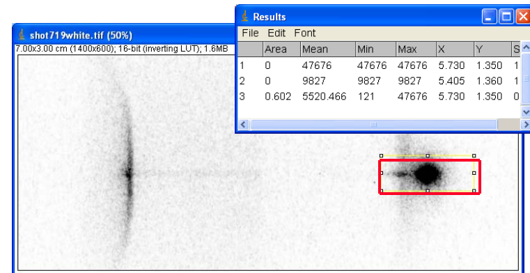
(4) Pre defined rectangle centered about spot1(Rod Pinch area) Peak Point and the mean is recorded
