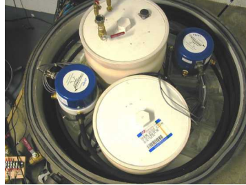
Figure 1 Sandia's acoustic test chamber (white dome), acoustic source and MB2000 (Left) and inside acoustic test chamber. Showing two CP 2.5 sensors, porous-hose and volume reducing fixtures (Right).
