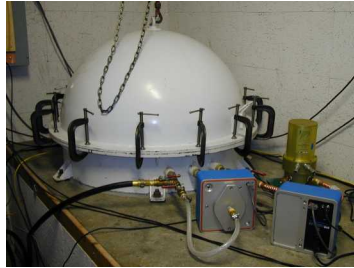
Figure 1 Sandia's acoustic test chamber (white dome), acoustic source and MB2000 (Left) and inside acoustic test chamber. Showing two CP 2.5 sensors, porous-hose and volume reducing fixtures (Right).
