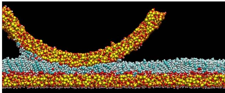
Rendering of simulations demonstrates, even with very low loads (<15 nN), coating material is transferred from the substrate to the AFM probe tip during shear.
