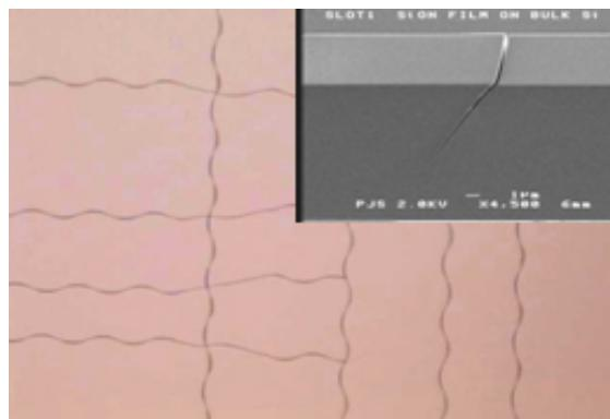
Optical film failure due to stress
