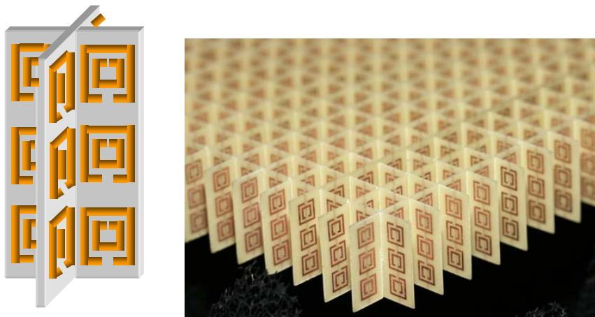
Split-ring resonator based unit cell forming a metamaterial structure
