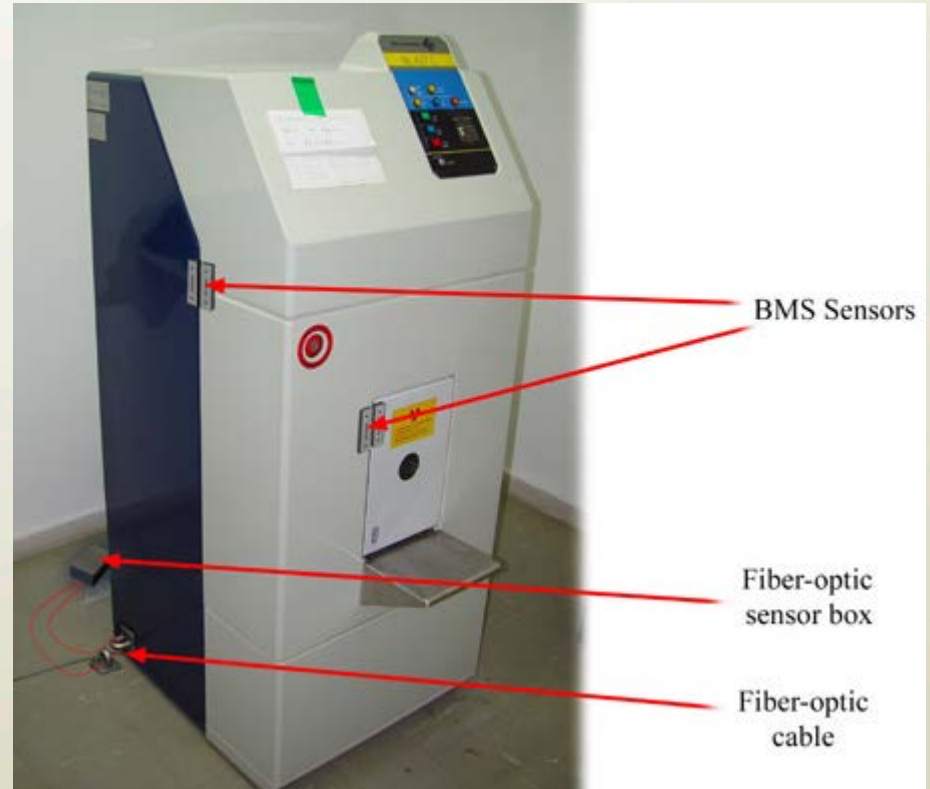
Blood Irradiator Unit. Sensor and fiber optic seal installed on each unit, so an alarm is triggered if an intruder attempts to remove the source.
