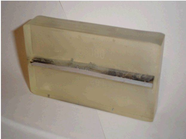
Figure 6. Test 1 prepped for SEM/EDS analysis
