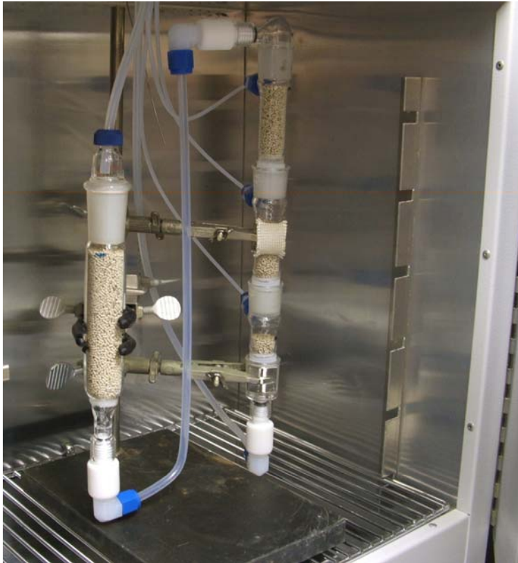
INL simulated dissolver off-gas setup
