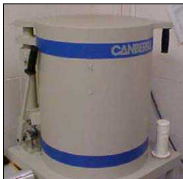
Gamma detector with Plexiglas sample holder to keep a uniform distance between the sample and the detector.
