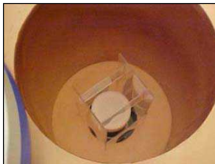
Gamma detector with Plexiglas sample holder to keep a uniform distance between the sample and the detector.
