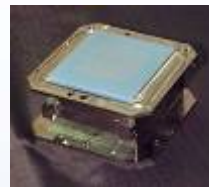
NUDET Sensors for satellite payloads (2000:1 size reduction)
