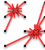
Figure 3b) Diagram of finding closest local cluster center in local k -means.
