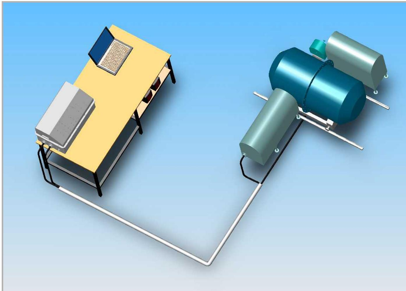
**The workstation and the measuring bench are connected via shielded cables.**
