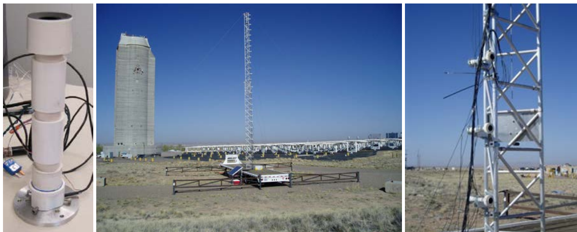
Figure 2: Left: Collimated LI-COR pyranometer [1]. Middle: Photo of trailer-mounted mobile heliostat target with NSTTF central receiver tower in background. Right: close-up of collimated pyranometers mounted on aluminum tower.
