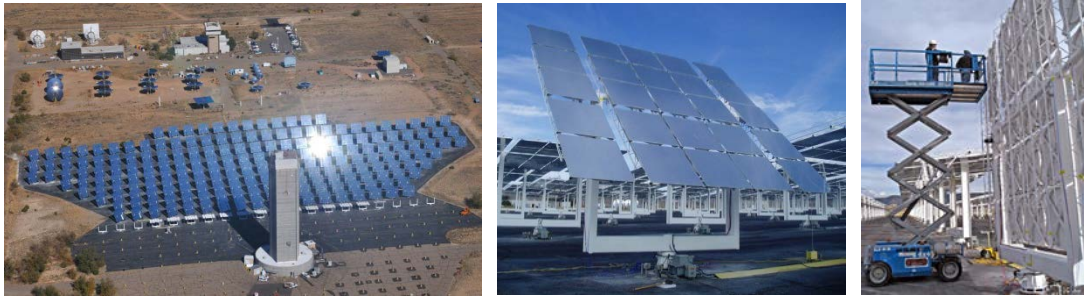
Figure 1. Left: Heliostat field at the NSTTF, Albuquerque, NM. Middle: Close-up of 37 m 2 heliostat. Right: Installing accelerometers and strain gauges on heliostat.
