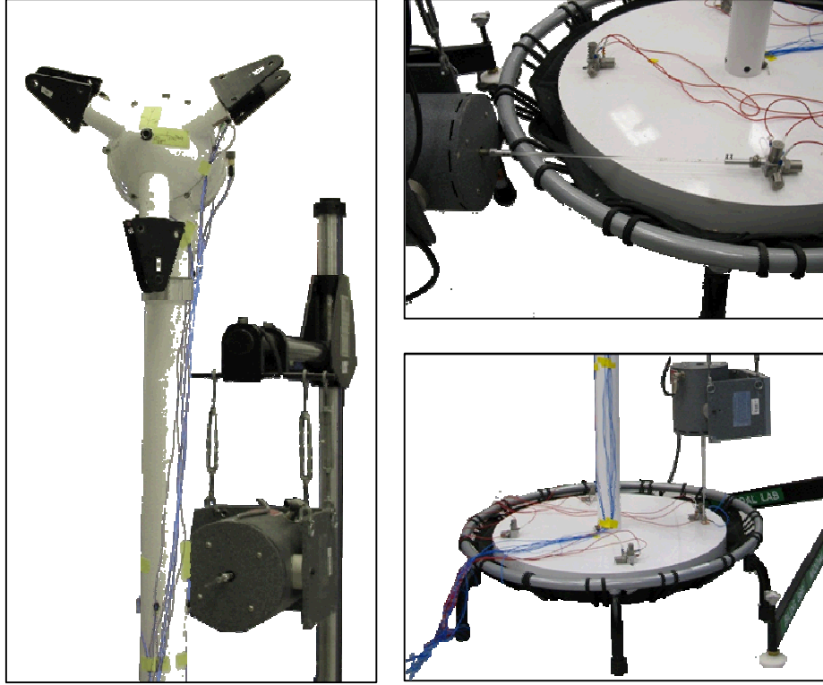
Figure 4: Drive points to excite rigid body modes: Tower for pitching and rolling modes (left) and base for yawing (top right) and -direction bounce (bottom right).
