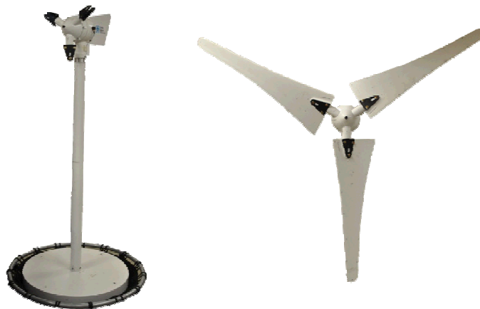
Figure 2: Structures tested to perform substructuring. (a) Bladeless tower (left) and (b) hub and blades (right)
