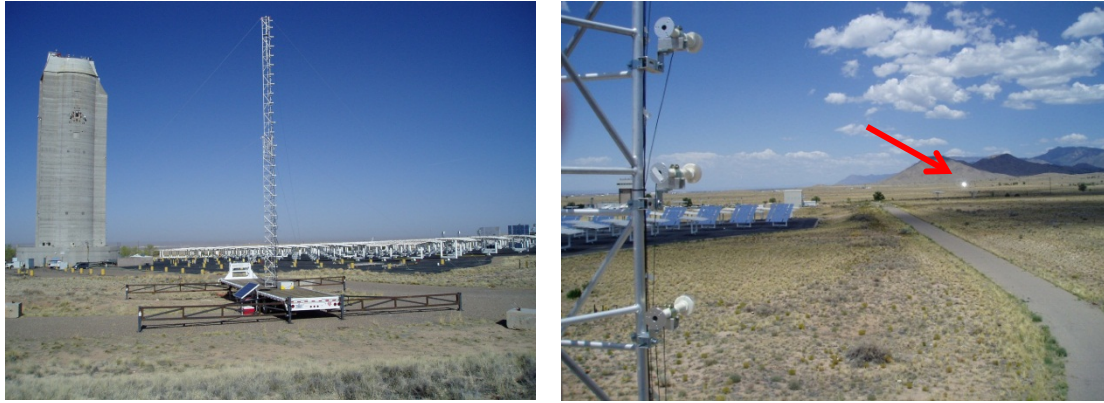
Figure 3. Left: Long-range heliostat target (LRHT) [2]. Right: View from the (LRHT) looking at the solar reflection from a single facet ~1700 m away.
