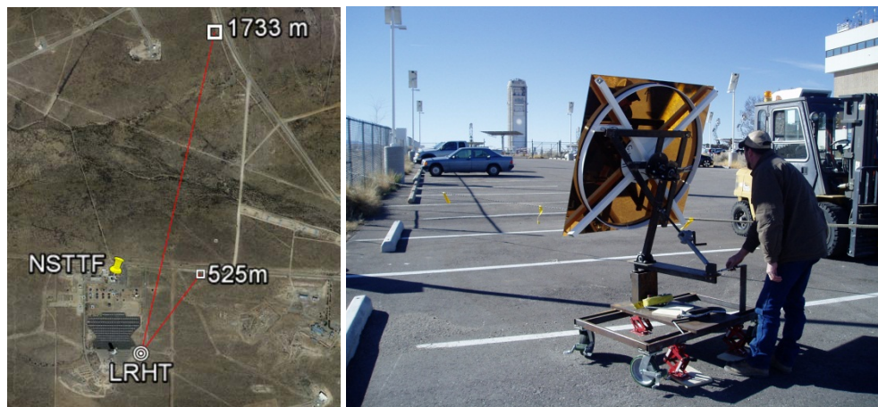
Figure 2. Left: Map showing the locations of the single-facet beam tests at 525 m and 1733 m away from the long-range heliostat target (LRHT). Right: Rig used to hold and track the facets.
