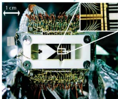
Demonstrated junction shuttling in 3 layer trap (~80% success rate)
