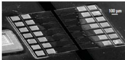
Lithographically fabricated GaAs trap, demonstrated at Michigan
