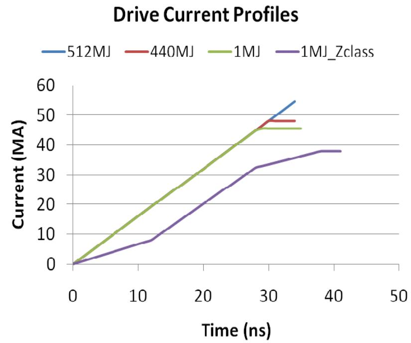
Producing  $dI/dt = 1.5 \times 10^{15}$  A/s in a 2.5 mm radius capsule requires a new technology.
