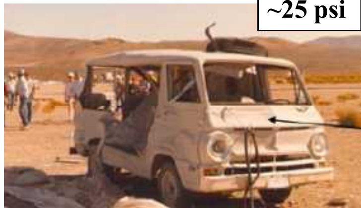
“Witness” vans at 30 feet from unmitigated and mitigated 100 lb detonations
