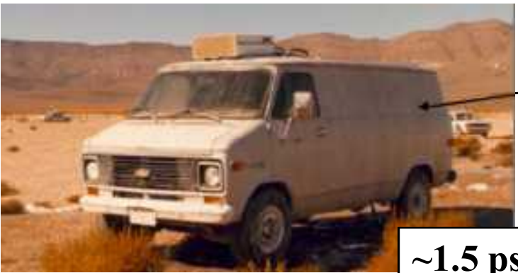
“Witness” vans at 30 feet from unmitigated and mitigated 100 lb detonations
