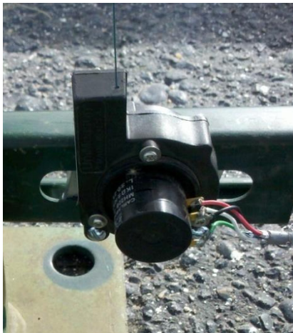
Figure 6: String Potentiometer Used in Displacement Testing
