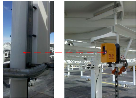
Figure 4: Ruler Displacement Method
