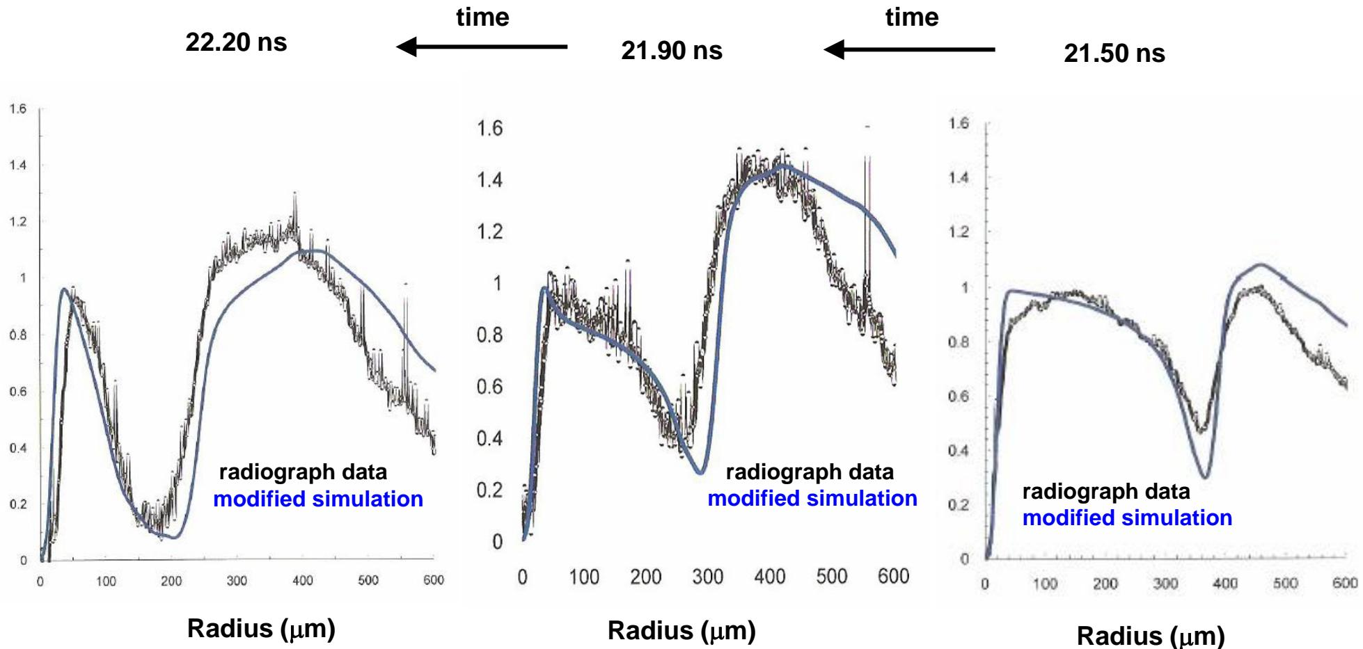
The radius, velocity, and remaining mass can be inferred from comparisons of the simulations with the radiograph data.
