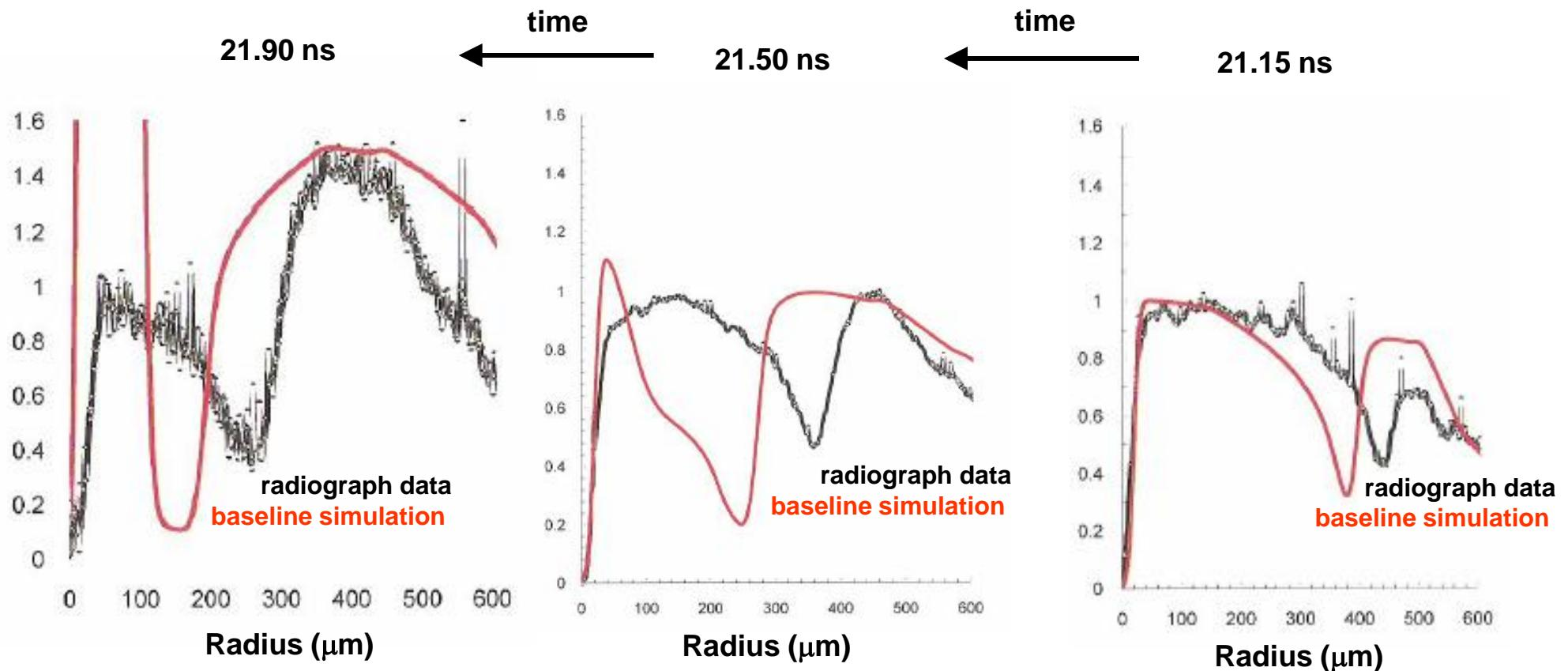
The modified (85% laser peak power) post shot simulation provides a reasonable match to the N110625 (Ge-doped CH capsule) radiographs.
