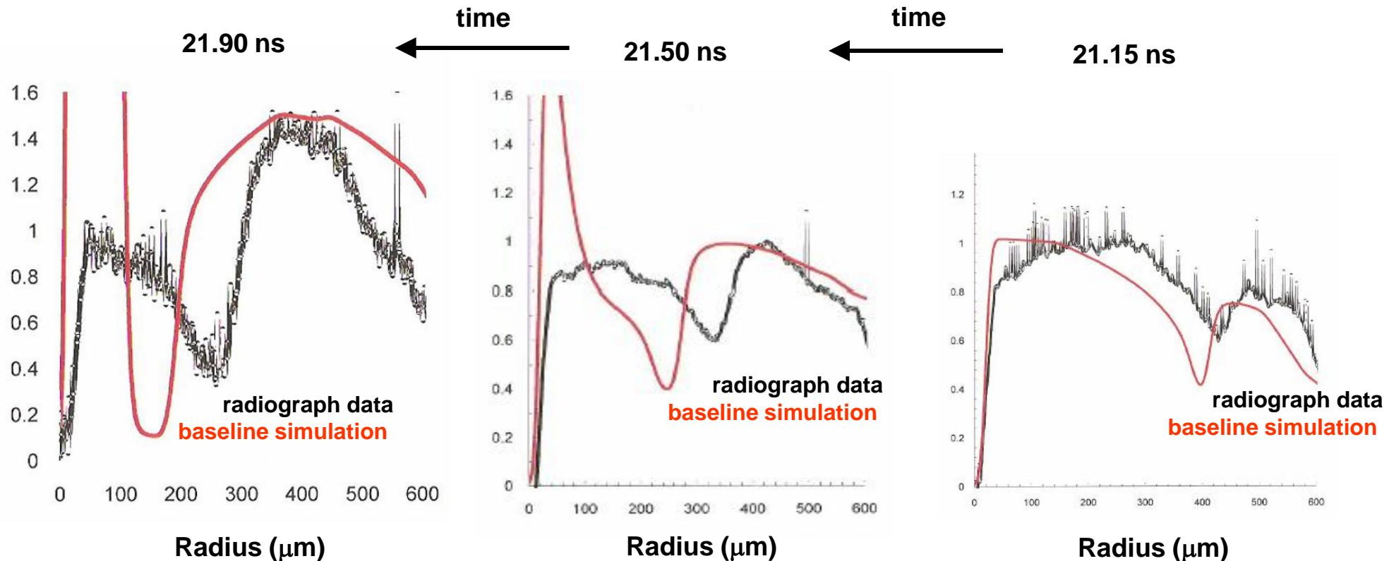
The modified (85% laser peak power) post shot simulation provides an improved match to the N110627 (Si-doped CH capsule) radiographs.
