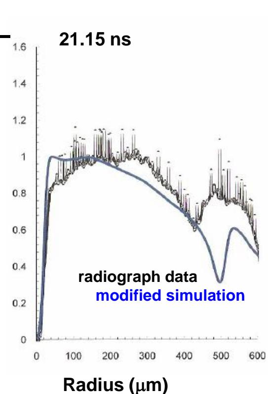
The radius, velocity, and remaining mass can be inferred from comparisons of the simulations with the radiograph data.
