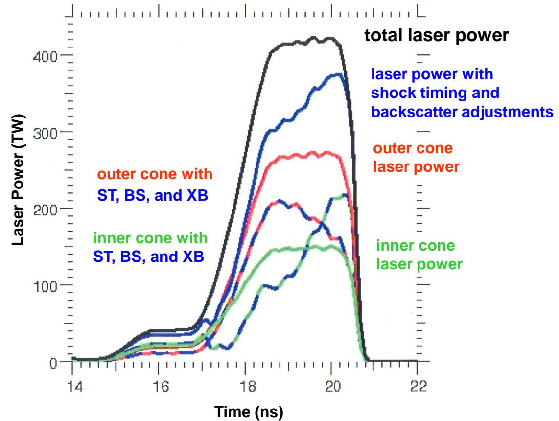
*The laser pulse shapes and absorbed laser energies are nearly identical for the Ge and Si doped CH capsule experiments compared in this presentation.*
