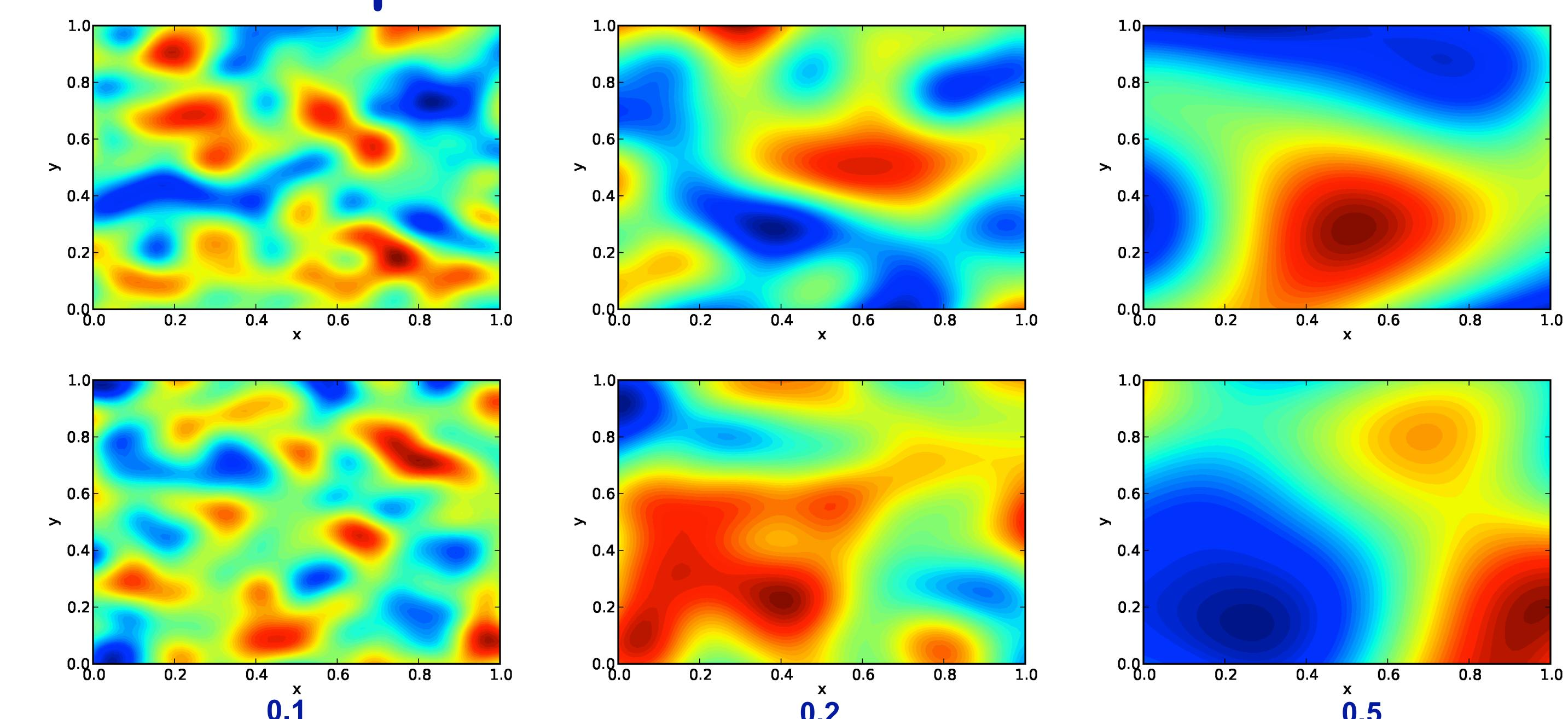
The Karhunen-Loeve expansion is used to generate realizations from a Gaussian random field over a range of correlation lengths. Two random realizations are shown for fields with correlation lengths of 0.1, 0.2, and 0.5, as indicated, highlighting the different range of length-scales in each case.
