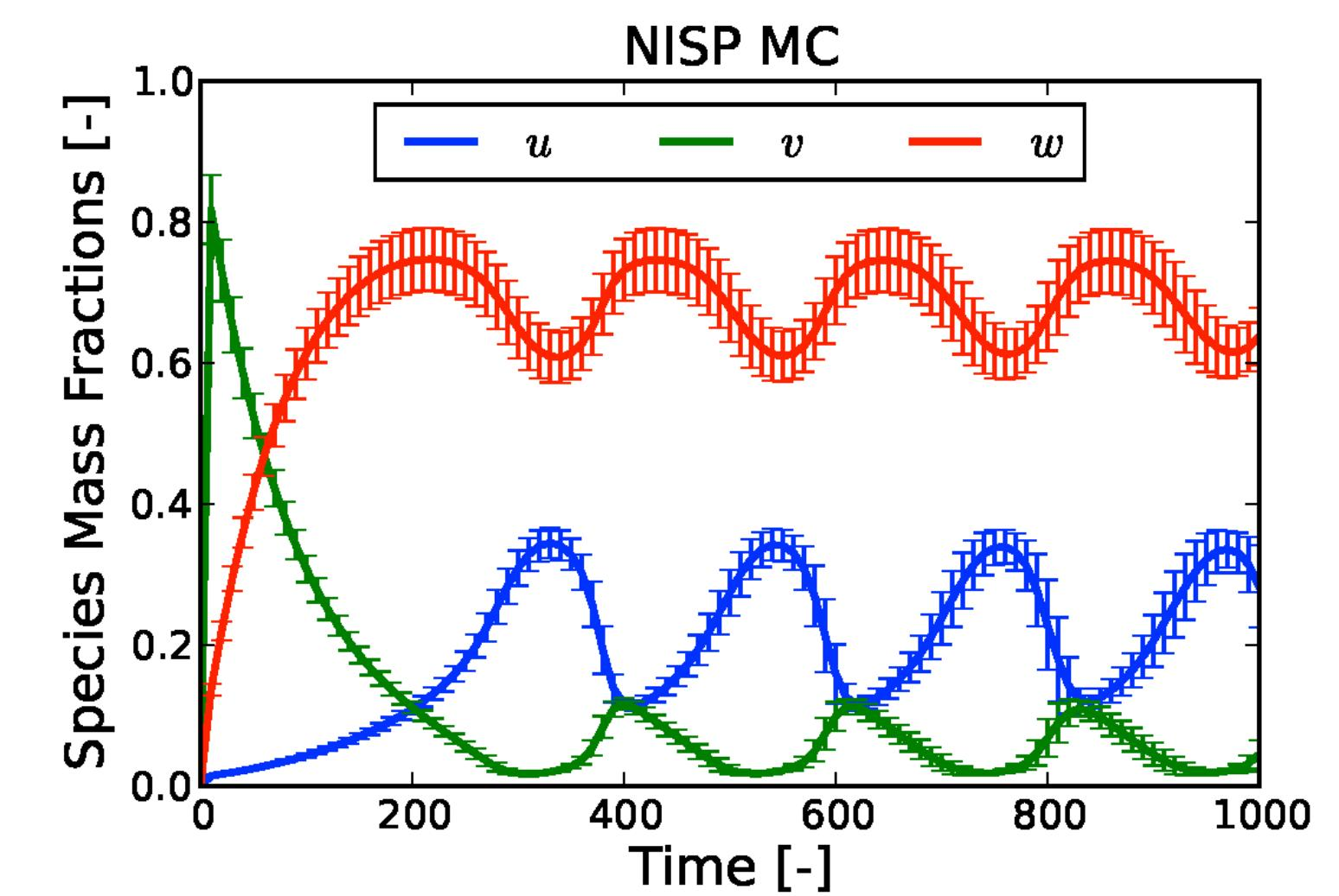
Non-intrusive Polynomial Chaos UQ application in a surface-reaction ODE model, with uncertainty in one chemical rate parameter.
