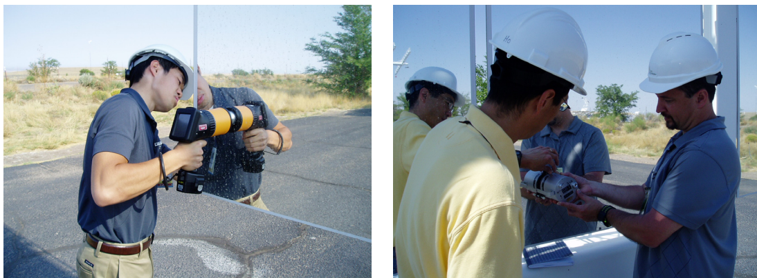
Figure 3. Reflectivity measurements of the SMF1100 facets on the 12W14 heliostat using the 410 Solar (left) and D&S 15R reflectometers.
