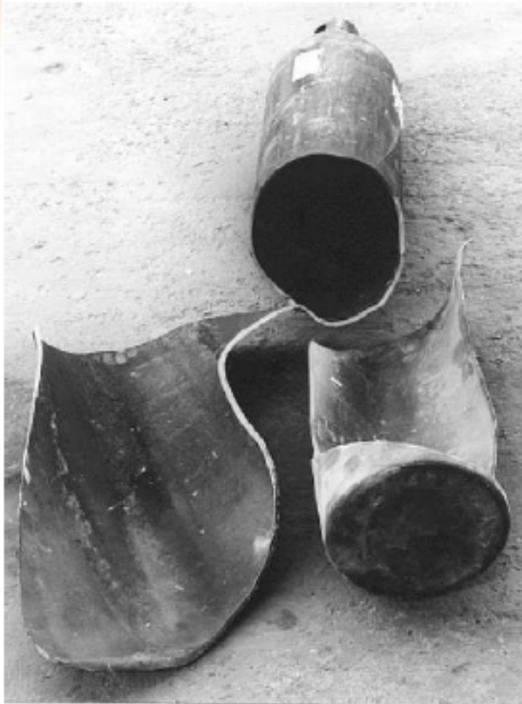
Hydrogen-induced failure of transport cylinder
