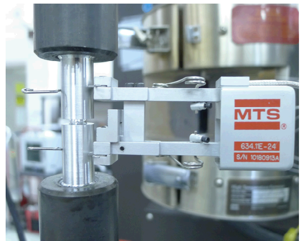
Figure 3 Tensile experiment setup.
