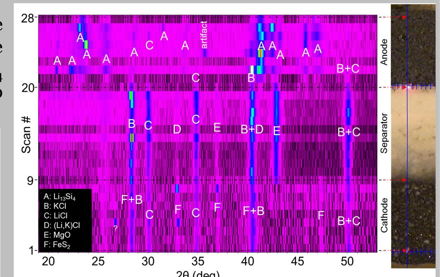
Standard XRD plots compiled are into a contour image to show the respective phases present as the thermal battery region is linearly spanned. Focusing on the anode region the primary phase observed is  $\text{Li}_{13}\text{Si}_4$  (label A).
