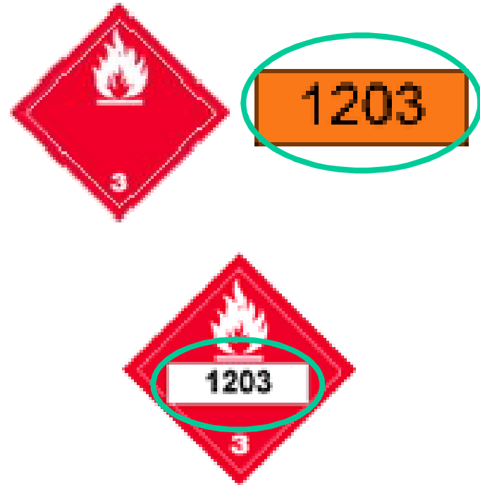
UN number and diamond label arrangements (1203 is gasoline)
