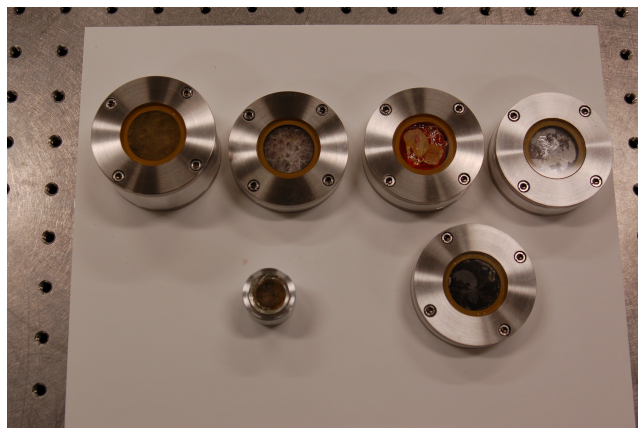
Fig. 1. Polycrystalline NaI(Li,Tl) samples tested for thermal neutron sensitivity. Diverse color and transparency can be seen in these samples, indicating the sensitivity of the material to variations in the production process and dopant concentration.
