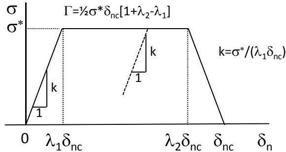
Plane strain cohesive zone model for mode I opening (when  $\delta_n < 0$ ; can define a multiple of  $k$  to penalize penetration)
