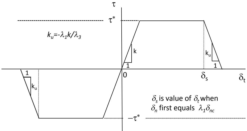
Plane strain cohesive zone model for mode II shear yielding prior to mode I softening (i.e., when  $\delta_n < \lambda_1\delta_{nc}$ ).
