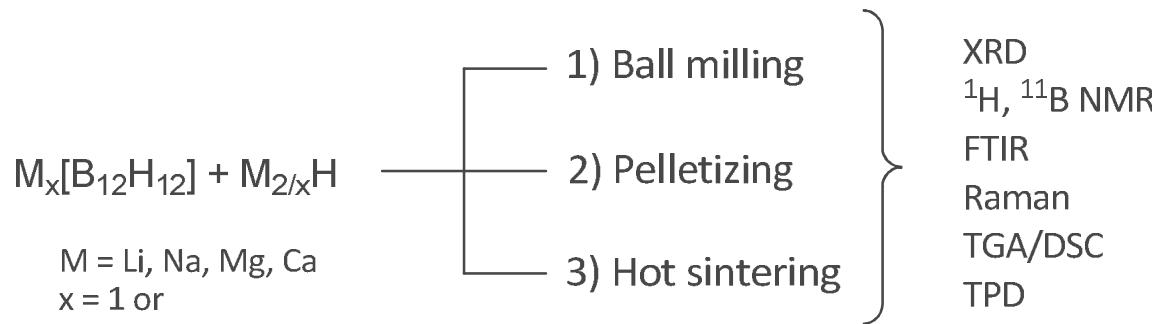
*Milling conditions* : high-energy, 30-120 min; *Pelletization* : 30 MPa, 5 min
