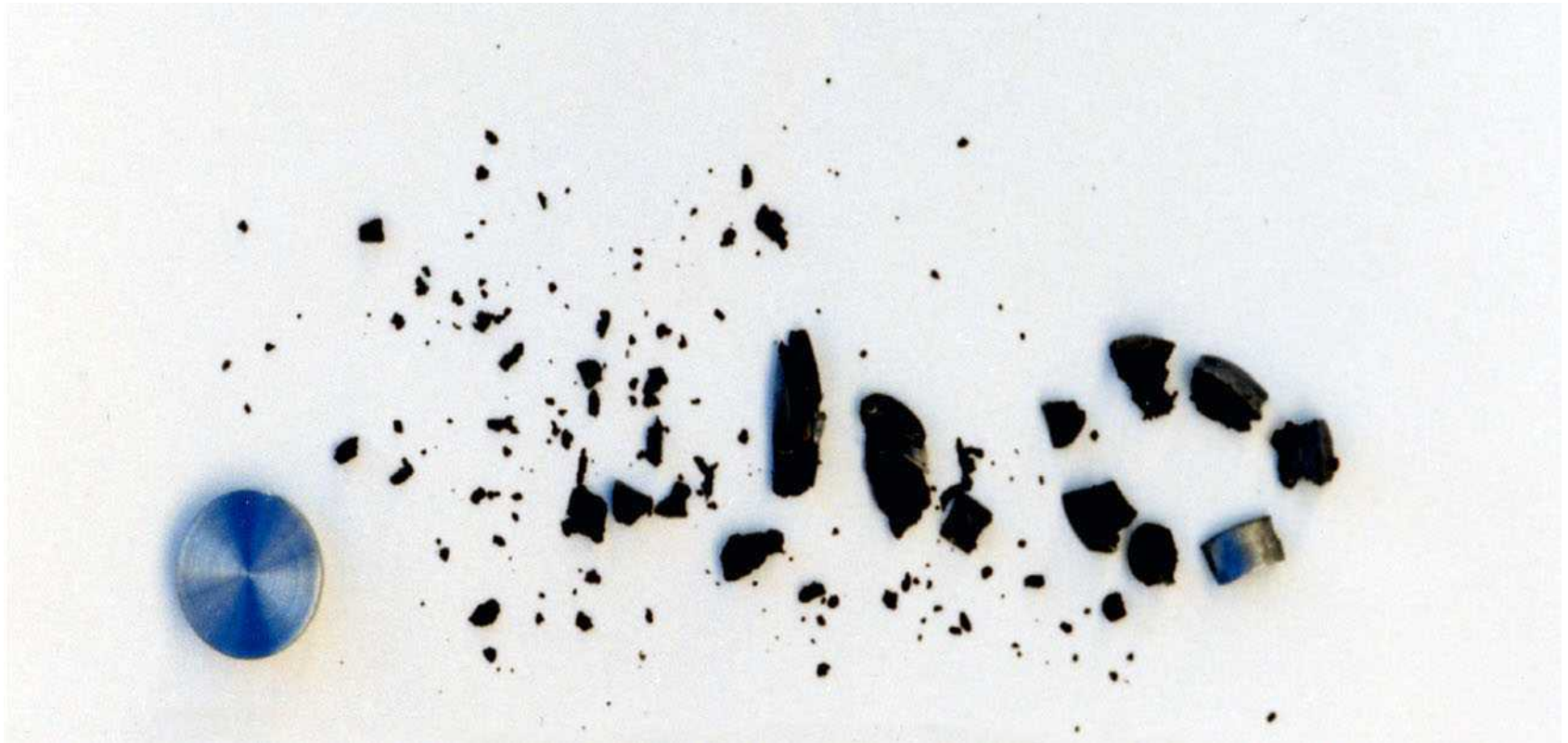
Before and After Witness Pellet Response to Simulated Lightning Pulse Into Conductors Adjacent to Insensitive High Explosives
