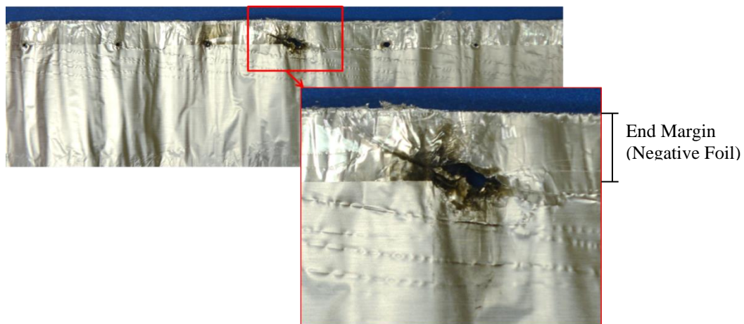
Figure 5. Crease-induced punch-through failure
