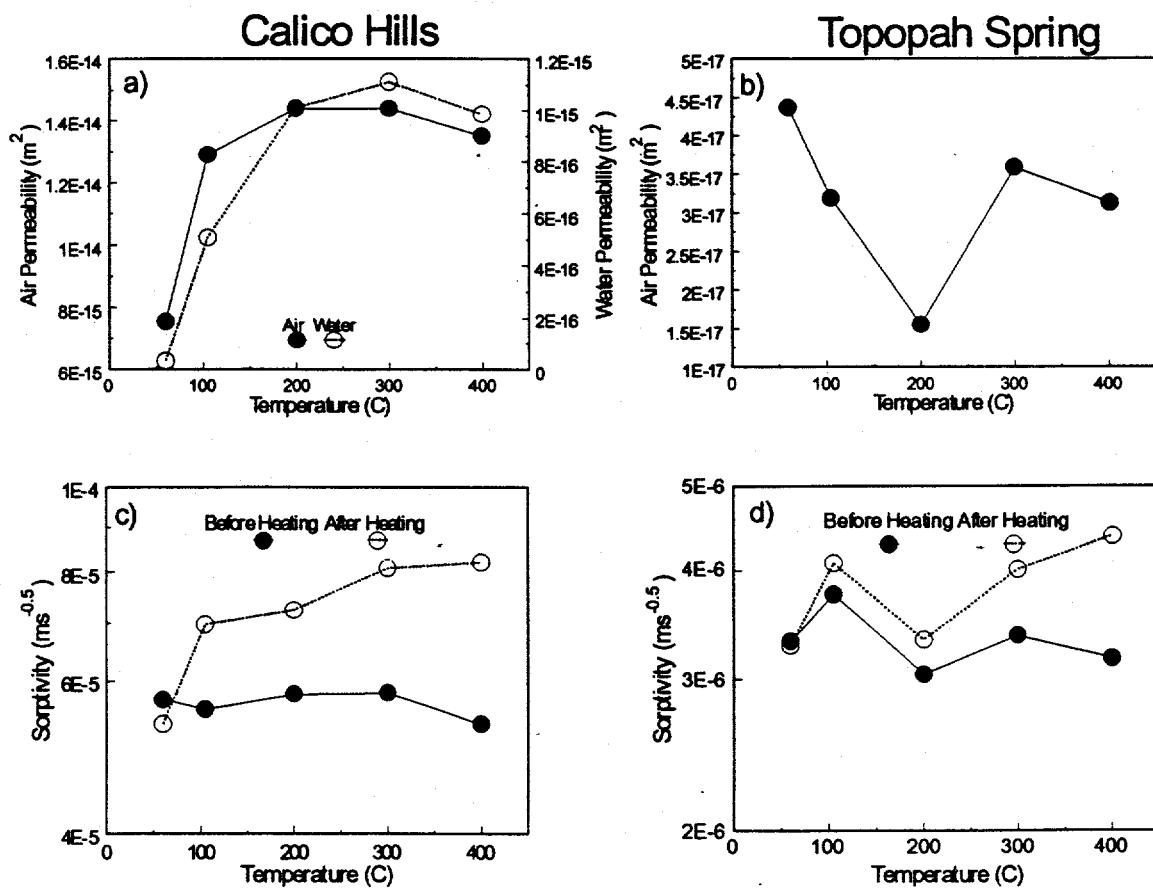
Figure 2. Change in the mean values of flow properties for samples dried at temperatures of 60, 105, 200, 300 and 400°C; a) nonwelded air and water permeability, b) welded air permeability, c) nonwelded sorptivity, and d) welded sorptivity.
