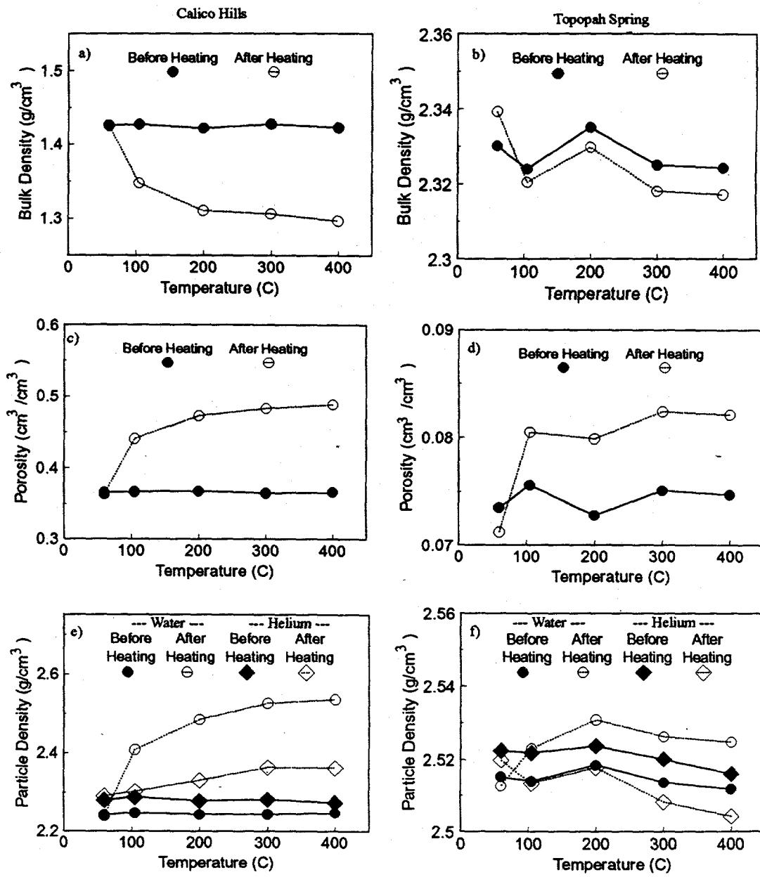
Figure 1. Change in the mean values of bulk rock properties for samples subjected to drying temperature of 60, 105, 200, 300 and 400 C; a) nonwelded bulk density, b) welded bulk density, c) nonwelded porosity, d) welded porosity, e) nonwelded particle density and f) welded particle density.
