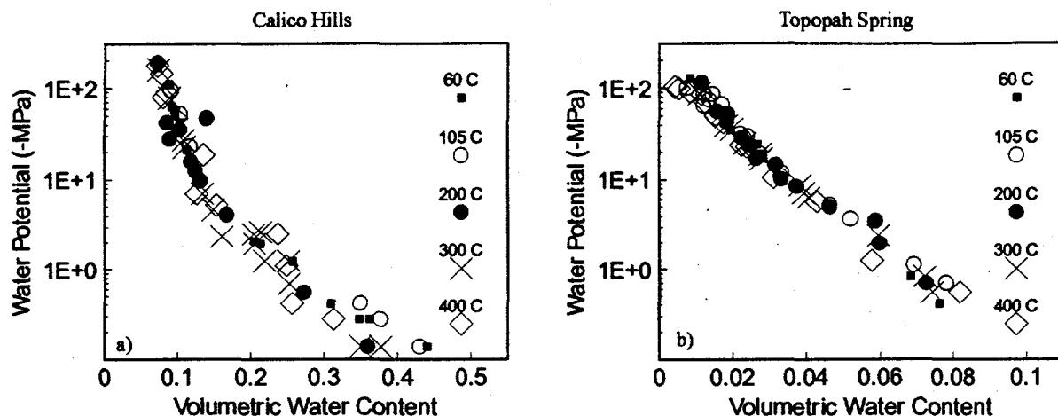
Figure 3. Water retention curves determined for core subsamples dried at 60, 105, 200, 300, and 400 C; a) nonwelded samples and b) welded samples.
