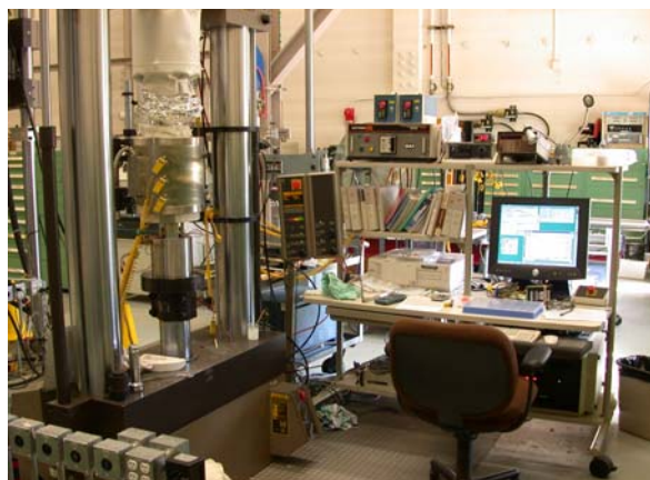
Fig. 4 Compression setup on 55.7 Kg (100 Kip) MTS test frame for intermediate temperatures.
