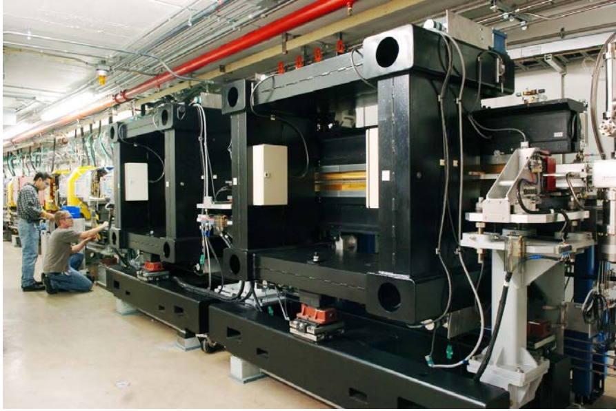
Figure 2: A canted, two undulator arrangement in the APS storage ring similar to that in the upgraded Sector 13. The downstream (right) device together with beamline optics provides X-rays in the 5-5-65 keV range to stations 13ID-C (interface scattering) or 13ID-D (laser-heated diamond anvil cell and large volume press). The photon beam from the upstream (left) device is canted outboard by 1 mrad and together with beamline optics provides X-rays in the 2.3-28 keV range for the X-ray microprobe in 13ID-E.
