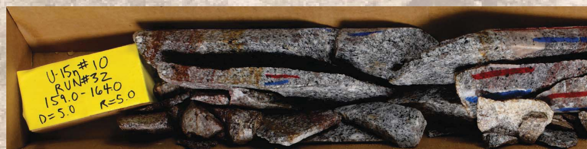
Photo of core recovered from angle-hole U-15n#10 near drilled depth of 159 ft. Fresh-looking fractures closest to yellow block are interpreted to be explosion-induced. SPE-N-2 source is approximately 4.5 m to the right. Yellow block is approximately 8 cm long.
