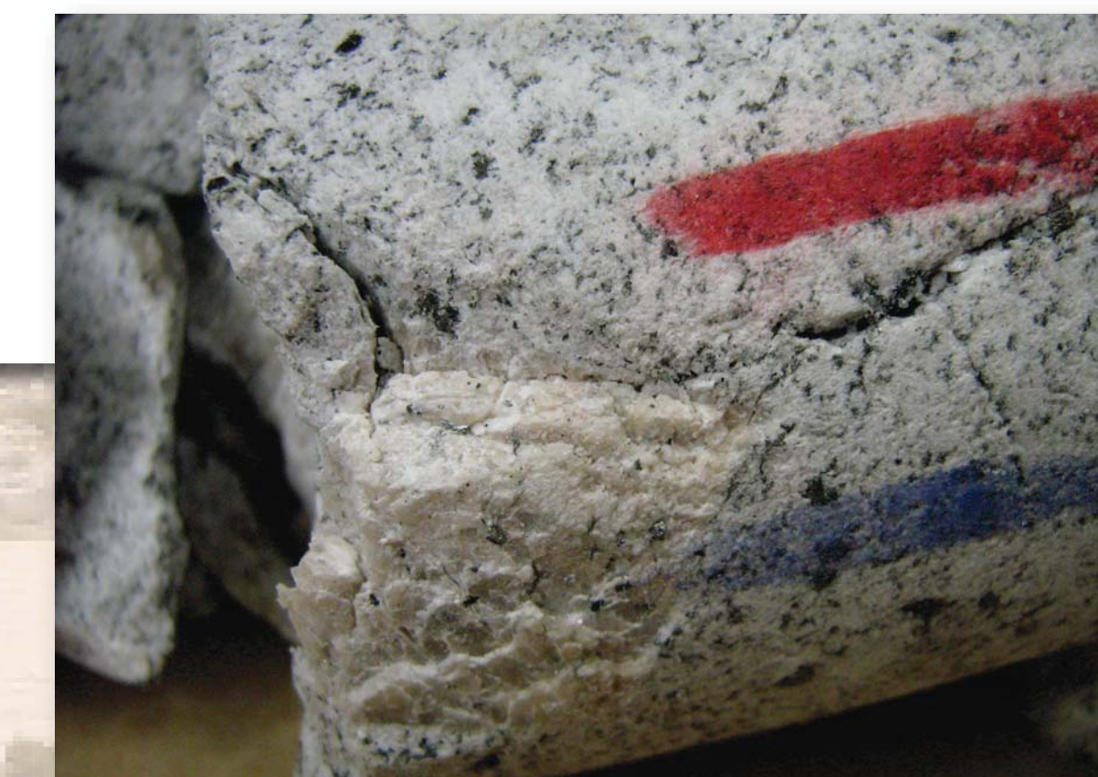
Fractured feldspar crystal retrieved from drilled depth of 168 ft in hole U-15n#10, approximately 1.8 m from the SPE-N-2 shot point. Red line is approximately 2.5 cm long.
