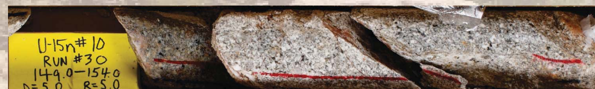
Photo of core recovered from angle-hole U-15n#10 near drilled depth of 149 ft. Note altered appearance of granite and coated fracture surfaces, indicating a natural fault. SPE-N-2 source is approximately 7.6 m to the right. Yellow block is approximately 8 cm long.
