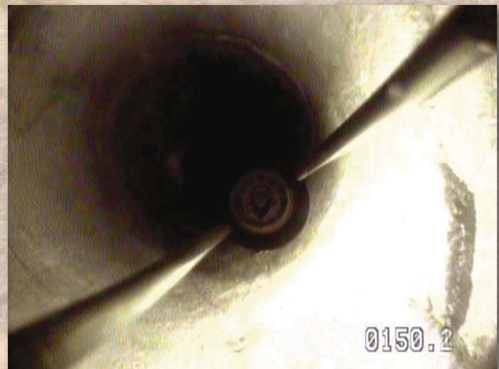
View of 0.91-m-diameter source hole prior to SPE-N-2, showing SPE-N-2 shot point location at a depth of 45.7 m. Note smooth borehole walls.
