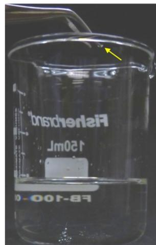
**Figure 3.10 Doping of Solution with Seed Crystal**
