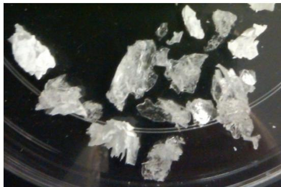
**Figure 3.8 Magnified Crystals from Rich PZ Solution**
