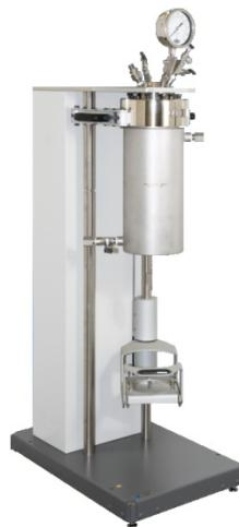
**Figure 5.6 Parr Pressure Vessel Assembly**
