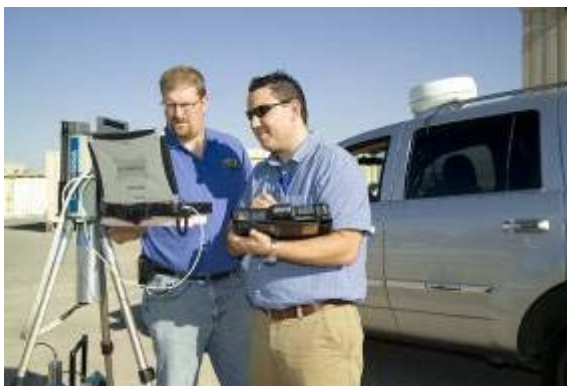
FIGURE E-4. DATA TABLET WITH MPCD EXTERIOR MODULE INSTALLED ON VAN
