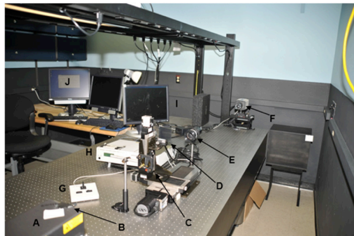
Fig. 2.5.1. Photograph of holography reconstruction bench here the image volume is reconstructed and converted into digital images.
