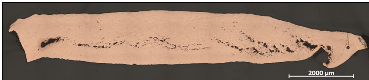
Figure 12. Cross section of the PBX 9501/copper sample showing clear evidence of damage. The feature at the right end is not seen in the radiograph and therefore was likely caused during the recovery process.
