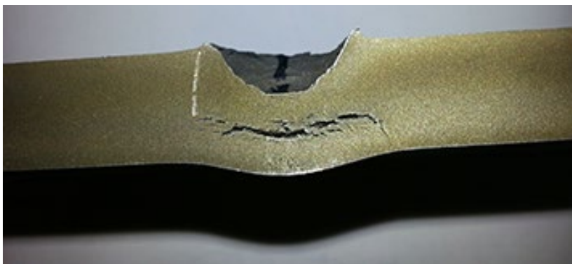
Figure 6. A sectioned target (Test ID 1000-016) plate confirmed spall fracture had occurred
