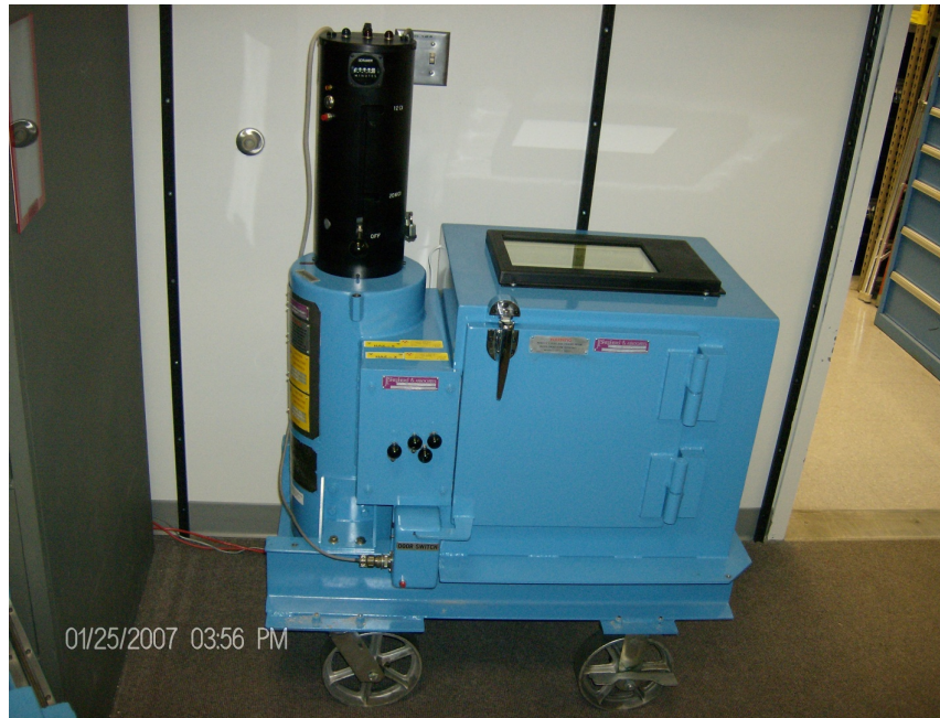
Figure 1: Shielded calibration range
