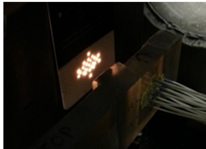
Typical 25-probe MPDV arrangement
